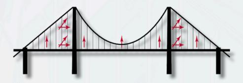
Typical example: An 1850m cable-suspension bridge spanning a critical harbor in Southern California. 26 strong motion accelerometers mounted on the bridge deck and base. Data monitored in real time in multiple locations.
