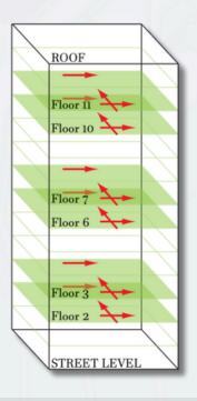
Example: 24-story steel frame building. Three uniaxial accelerometers per instrumented floor (two E-W, one N-S) are deployed at nine floors plus the roof. Inter-story drift ratios calculated, thresholds aligned to design criteria, and events auto-reported to stakeholders via web/SMS/email.
